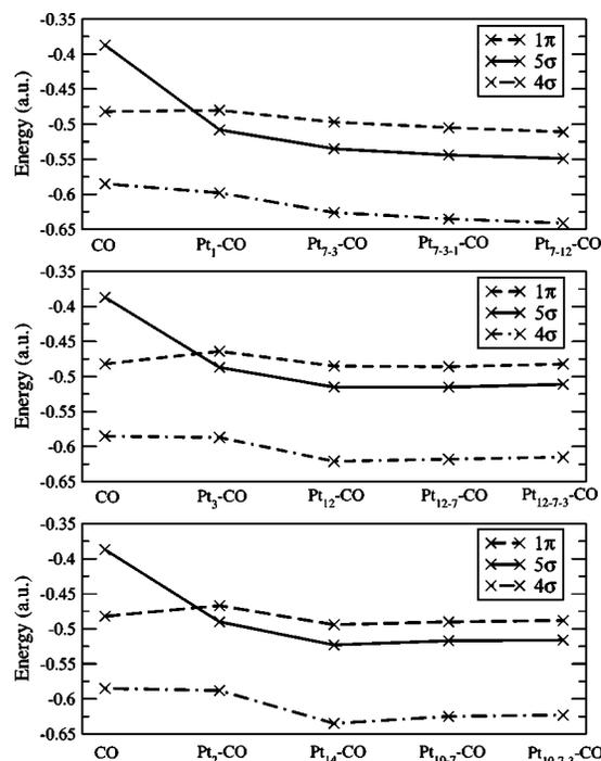
FIG. 2. Variation of the 4σ, 1π, and 5σ orbital energies. Top panel, on-top binding site; middle panel, threefold binding site; and lower panel, bridge binding site.
