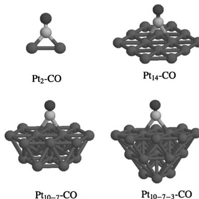
FIG. 5. Cluster models of the twofold (bridge) binding site.
